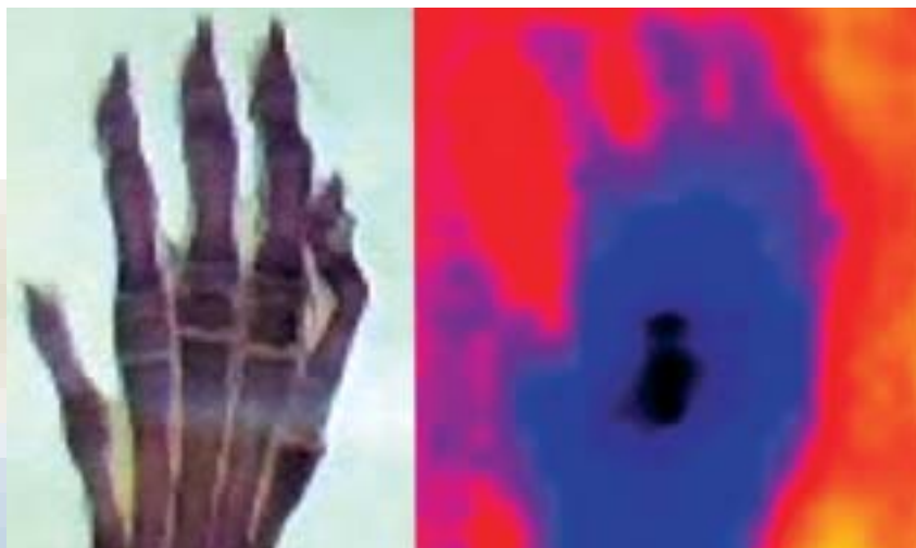
An x-ray of a rat's paw (left) and a false-coloured image created by neutron absorption
